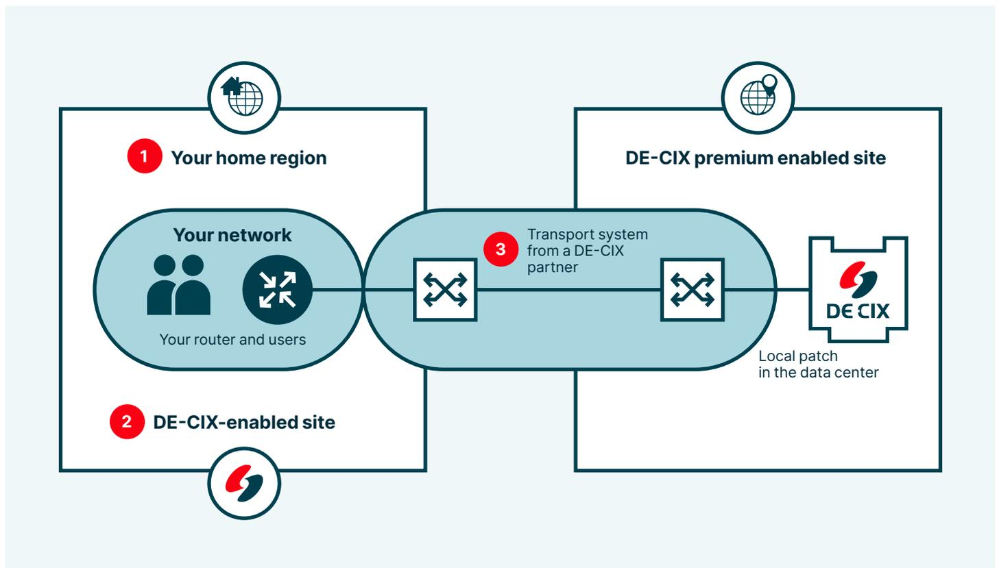
→ It is the same setup as a classic connection to DE-CIX – just without having a router at a DE-CIX premium enabled site but instead at a DE-CIX-enabled site.
